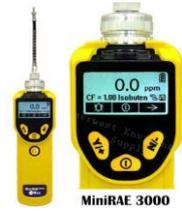
The portable pid is used for hydrocarbon monitoring. It uses light to ionize hydrocarbons and detects them
