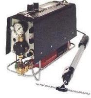
The portable fid is often seen as the field work horse for hydrocarbon monitoring. It allows the operator to build a quick picture of the total hydrocarbon count in the immediate environment
